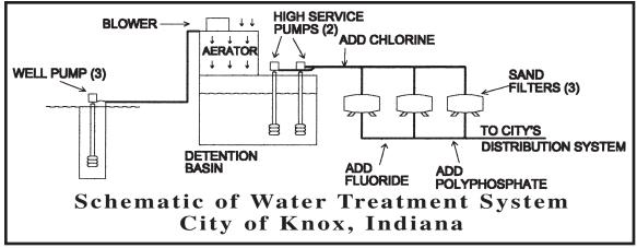
pumps, called high service pumps, move the water from the detention basin through pressure sand filters completing the iron removal process. Chlorine is added prior to the pressure sand filters for disinfection. The water leaving the filters enters the water distribution system after receiving fluoride and polyphosphate addition and flows to the homes, businesses and industries of Knox.
